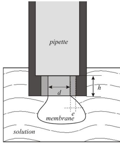
Furthermore, there is a junction resistance, which we need to take into account, it is called *seal* resistance and it is influencing the stability of the pipette-membrane circuit. This resistance is due to a cylindrical pillar surrounding the CZ of the same conductivity  $\sigma$  as the CZ. The thickness of this pillar is  $e = 3 \times 10^{-10} m$  ( $e \ll d$ ) and height  $h = 2\mu m$ .
