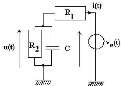
We consider the circuit shown here, consisting of a capacitor with capacity  $C$ , initially discharged, of two resistances  $R_1$  and  $R_2$ , powered by a generator delivering a variable signal  $v_e(t)$ .
