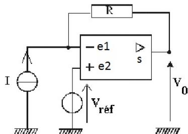
The operational amplifier (OA) is considered to be ideal and operating in linear regime. Under those conditions the AO behaves in the following way:  $v_{e1} = v_{e2}$  - the potential at input 1 is equal to the potential at input 2, and  $i_{e1} = i_{e2} = i_s = 0$ , the currents at the inputs and the output are all equal to zero. On the schematic we see a source of voltage and a source of current.
