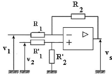
8. Express the output tension  $v_s$  as a function of  $v_1$  and  $v_2$  as well as the different resistances. The circuit considered in this question is shown above.
