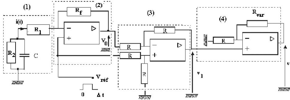
We model the equivalent resistance of the pipette by  $R_1$ , while  $R_2$  and  $C$  are representing the resistance and the capacity of the membrane (bloc1):
