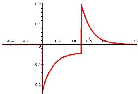
22. Using the collected data of  $v(t)$ , which is given below (the horizontal axis  $t$  is in seconds and the vertical axis  $v$  is in volts), find the values of  $R_1$ ,  $R_2$  and  $C$ . For those measurements we also know that  $V_{ref} = 5mV$ ,  $R_f = 100M\Omega$  and  $R_{var} = 0$ .
